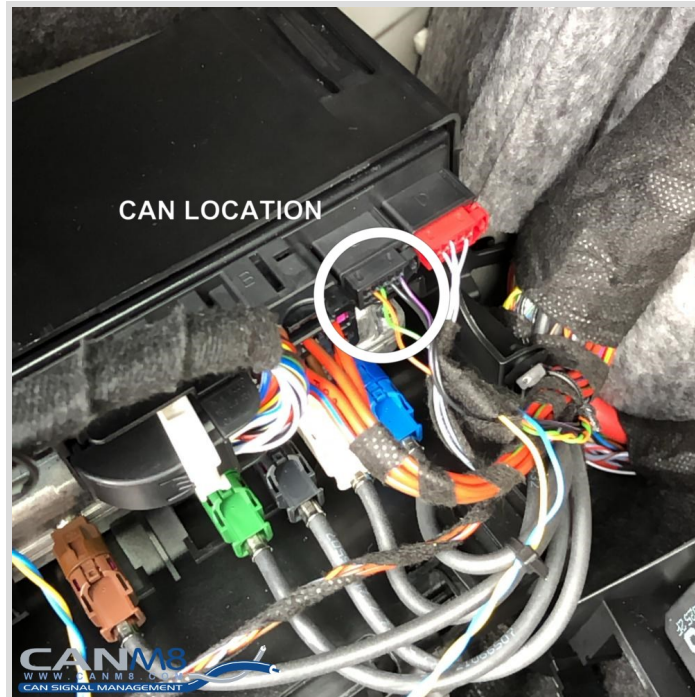
CAN wiring behind the left cover in the luggage compartment
